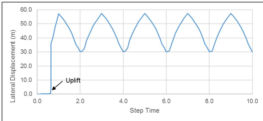
**Figure 14 Lateral Displacements of Pipeline at Channel 4 Under Cyclic Turbidity Current Loading**
