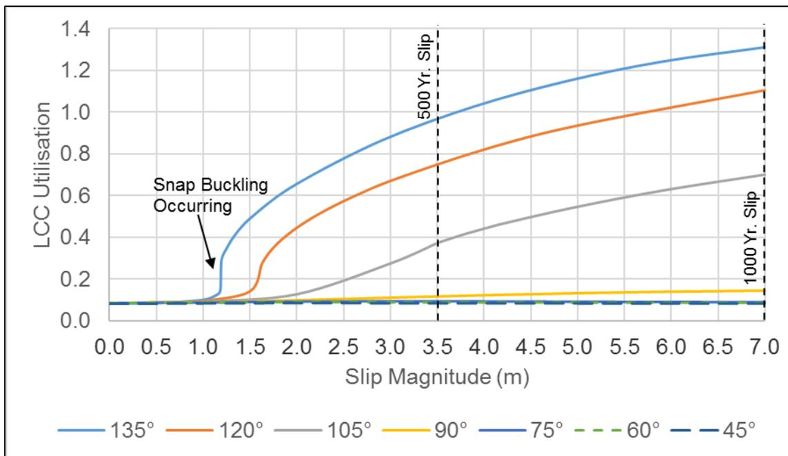
Figure 3 DNV Utilisation Versus Fault Crossing Angle
