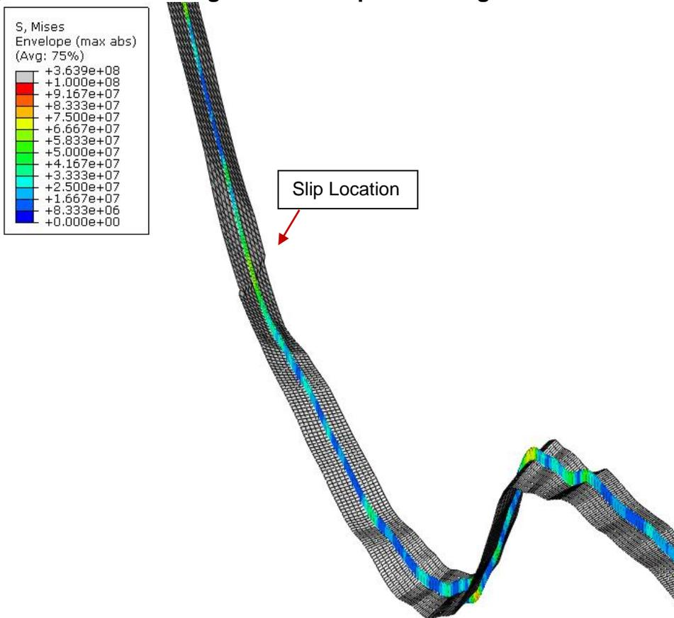
Figure 7 Fault Crossing Profile in Abaqus Showing von Mises Stresses
