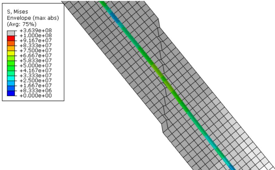
Figure 6 Fault Crossing Plan in Abaqus Showing von Mises Stresses
