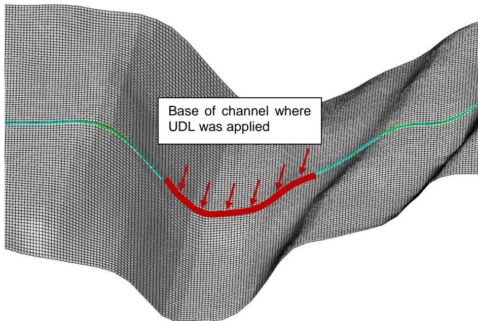
**Figure 12 Canyon Feature 4 Under Operational Conditions Showing Location Turbidity Currents Were Applied**
