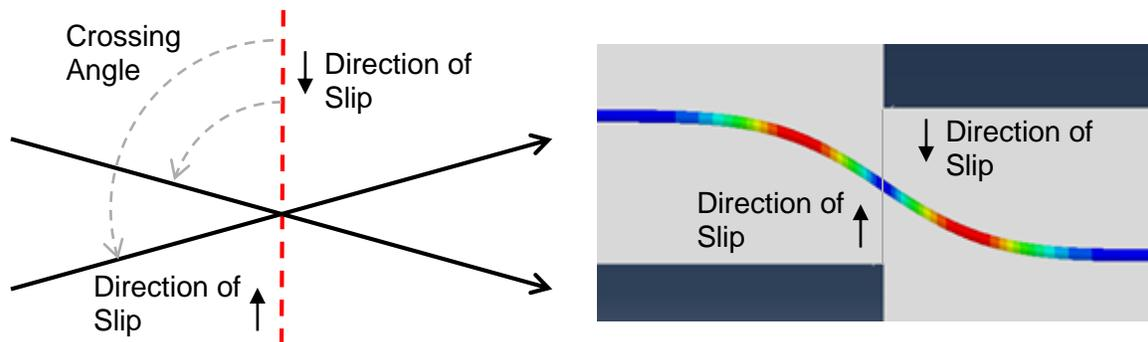
Figure 2 Fault Crossing Schematic and Abaqus Model
