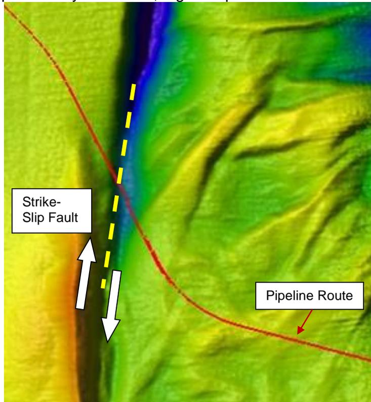
**Figure 4 Fault Crossing Plan**
