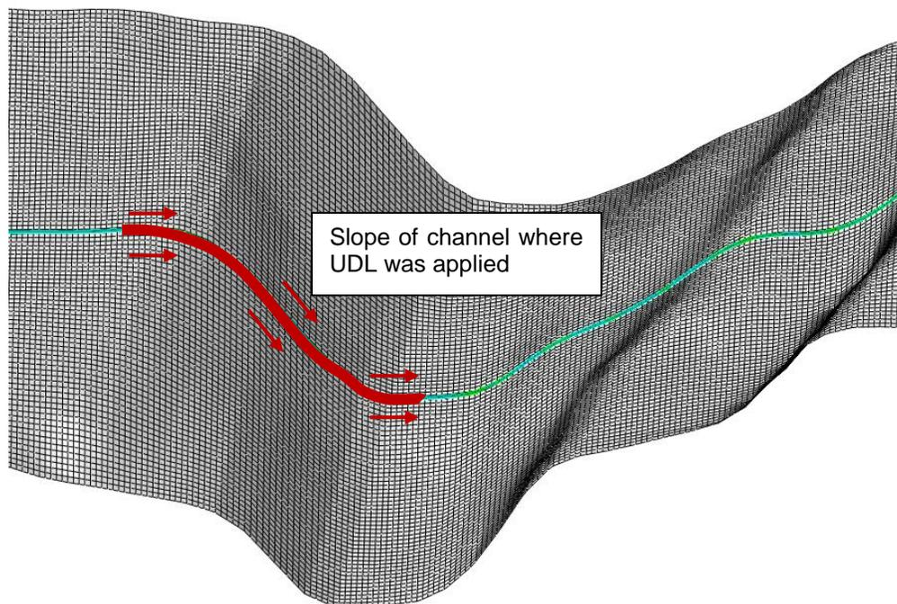
**Figure 15 Canyon Feature 4 Under Operational Conditions Showing Location Debris Flows Were Applied**
